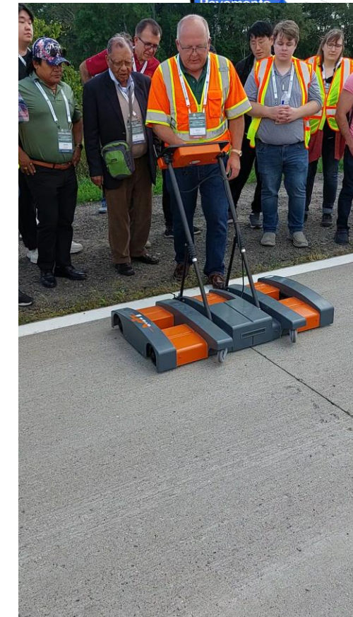
Site visit MnRoad test facility, with demo of MIT-scan
